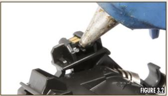
Install a new Static Control chip and secure with a small amount of hot glue, as shown in Figure 3.2.
