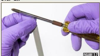
Holding the mag roller above the powder as shown in Figure 2.7, lightly tap the drive journal to dislodge any excess powder back onto the paper.
