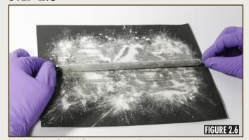
Holding the Static Control mag roller by the ends, slowly roll the mag roller back and forth through the powder until the mag roller is evenly coated (Figure 2.6).
