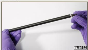
Install the mag roller magnet into the mag roller, leaving the keyed end of the magnet slightly extended out the end of the roller (Figure 2.9).
