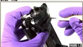
Gently and firmly pry up on the gear side end plate using a small slotted screwdriver to break the plastic weld, as shown
