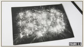
Apply a light, even dusting of Developer Roller Powder to a sheet of paper as shown in Figure 2.5.
