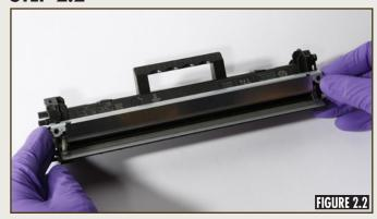
Place the doctor blade onto the toner hopper and install the two screws, but do not tighten them (Figure 2.2).
