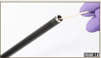
Apply a small amount of conductive lubricant to the interior of the mag roller using the wooden end of a cotton swab (Figure 2.8).
