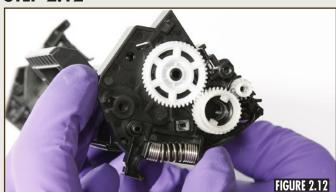
Install the mag roller drive gear, the agitator drive gear and the main drive gear as shown in Figure 2.12.
