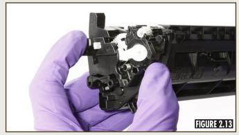
Install the gear side end plate and secure with two screws using a standard Phillips screwdriver (Figure 2.13).
