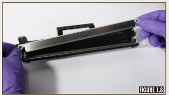
Remove the two screws from the doctor blade using a standard Phillips screwdriver and lift the doctor blade from the toner hopper (Figure 1.8).
