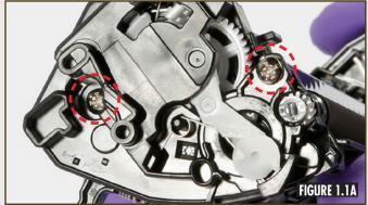
Use a standard Phillips screwdriver to remove the two screws in the gear side plate (Figure 1.1A).
