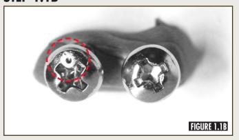
Note: Look closely at the screw heads for a dot (see Figure 1.1B), which indicates the screw has a left hand thread. No dot indicates a screw with the standard right hand thread.
