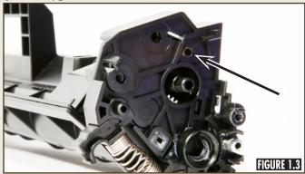
Remove the three (3) gears from the drive side of the outer hopper, set them aside and use the REPBIT-48 to drill a small hole in the inner end plate as shown in Figure 1.3.
