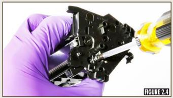
Install the contact side end plate and secure it in place using a replacement cartridge screw and a small Phillips screwdriver (Figure 2.4).
