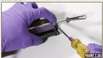
Using a feeler gauge as shown in Figures 2.3A and 2.3B, press down to set the height of the doctor blade and tighten the two screws.
