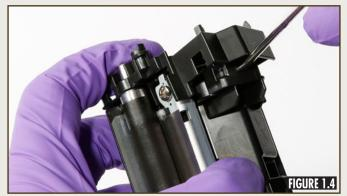
Using a small slotted screwdriver in the area shown in Figure 1.4, gently pry up to break the plastic weld and remove the inner end plate.
