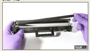
Grasping the mag roller by the drive journal, lift the mag roller up and out of the toner hopper (Figure 1.5).
